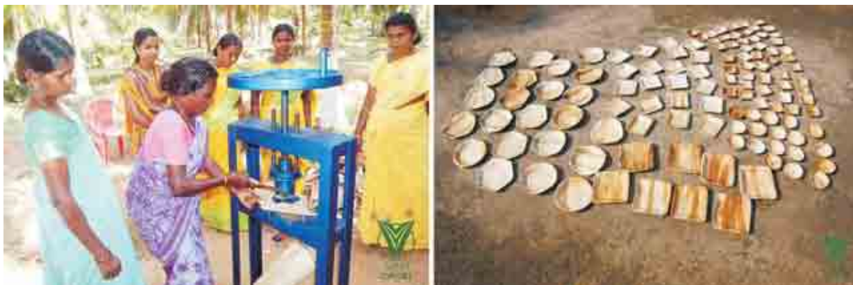
Utilization of arecanut leaf sheaths for production of eco-friendly plates and cups.
